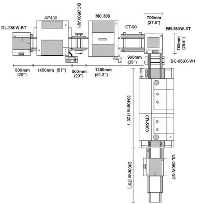
Figure 4: Line drawing example for tight space utilization.
