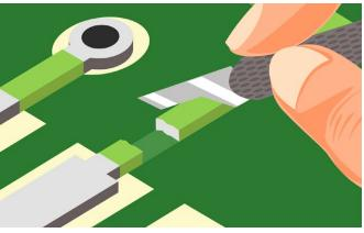
Figure 2: Use a sharp-edged knife to make the trace cuts.
