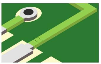
Figure 1: Determine the trace cut location.
