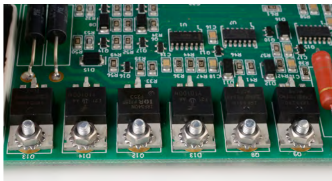
ParyFree coated and uncoated board after salt-fog testing.
